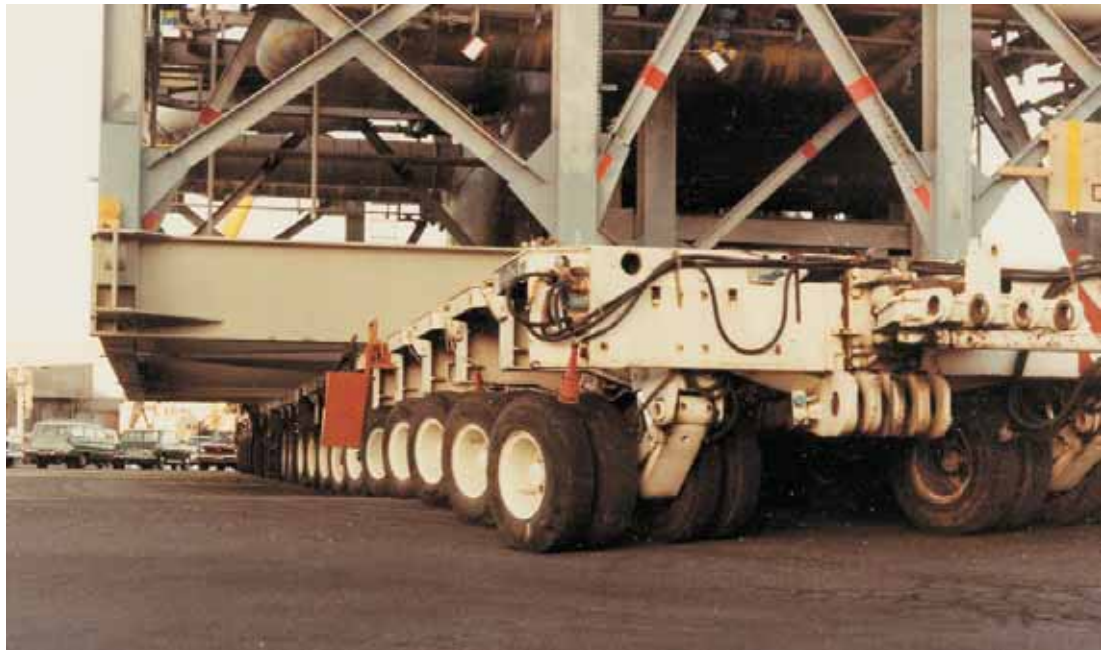
Figure 4: The 622P trailer traverses the Port silo corner - the uneven road profile results in full extension and compression of the hydraulic rams
